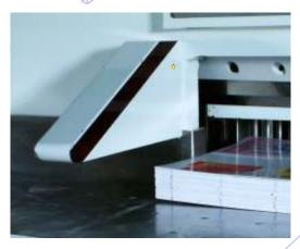
As per Safety standard it is not advisable to operate Paper cutting machine without Photo Safety. **The 'MICROCUT'** Paper Cutting Machine equipped with Two row of infrared safety barrier with row selection facility in front of cutting area to avoid accident which ensure safety at all the times while fault in one row.
